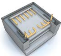
Section through the oven – steam distribution system
